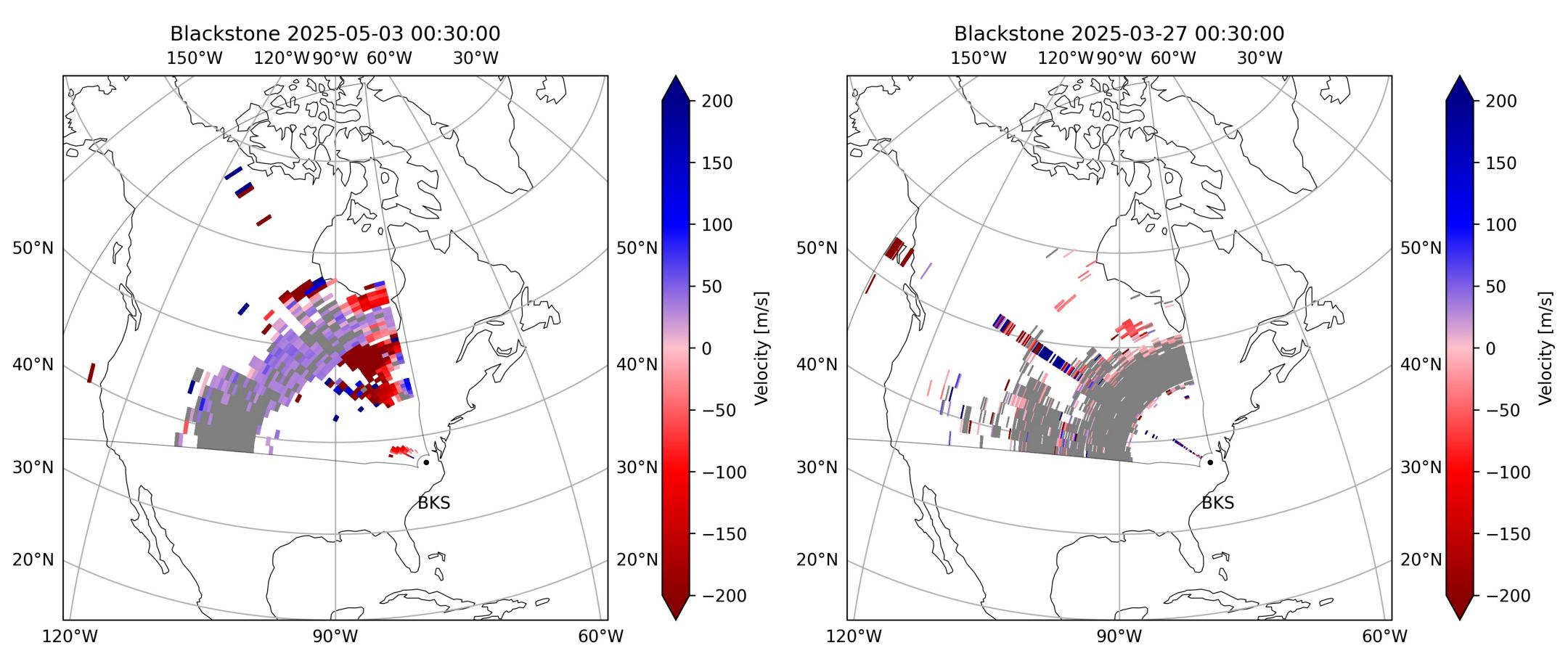
Fan plots displaying range gate differences between an unmodulated pulse (left, 45km range resolution) and a PCM pulse at 5-baud (right, 15km range resolution). Plots created using VT SuperDARN's online interactive fan plotting tool.
