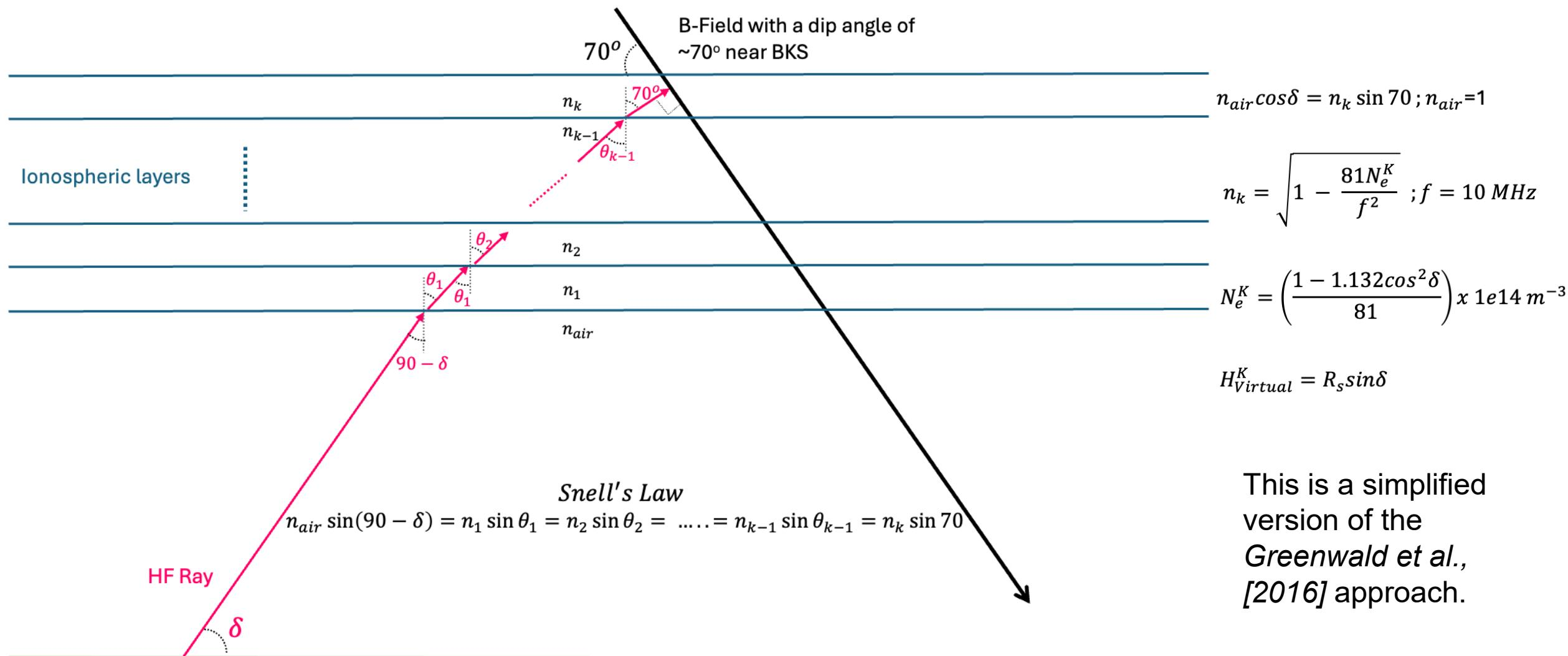
Using Snell's Law, we can estimate the electron density of the layer (here  $k^{\text{th}}$  layer) where the ray turns perpendicular to the B-field. The virtual height of the  $k^{\text{th}}$  layer can be estimated from slant range and elevation angle.
