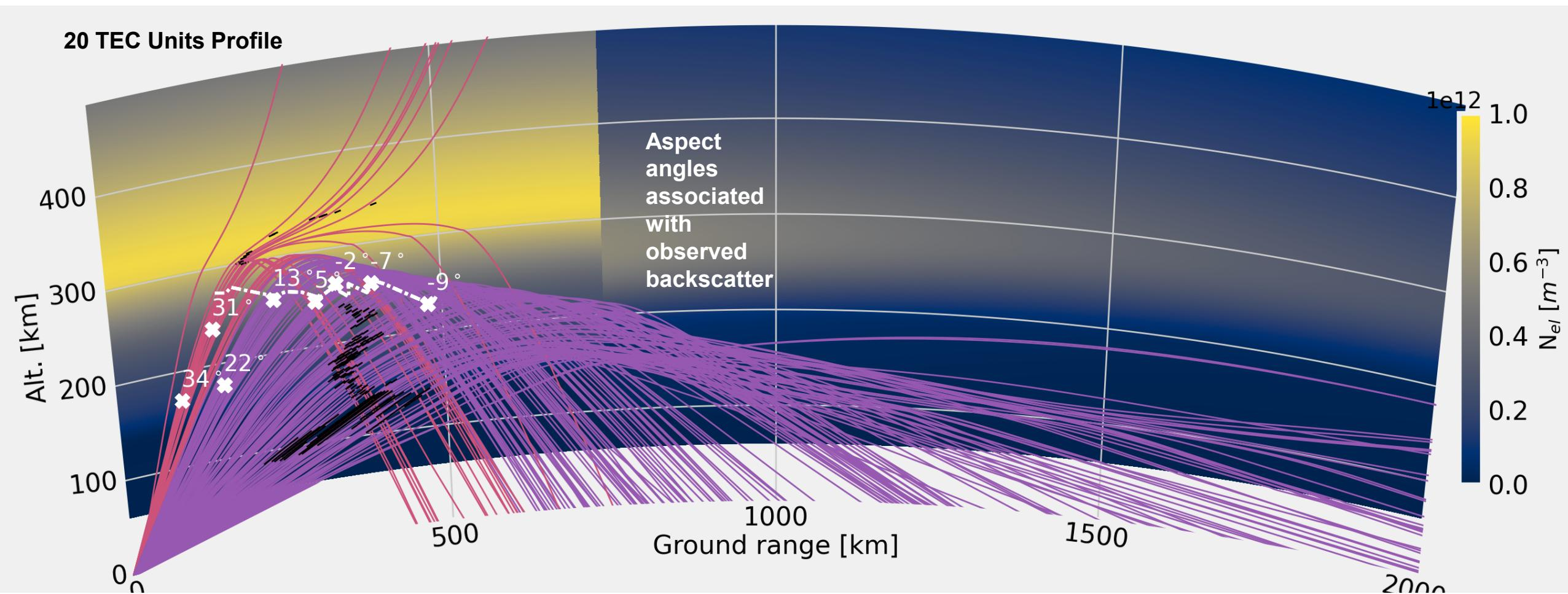
Ray-tracing through the *Fang et al., [2010]* profile suggests that the backscatter likely is originating between 250 and 300 km altitude, and also suggests that the denser ionosphere can produce ground backscatter.
