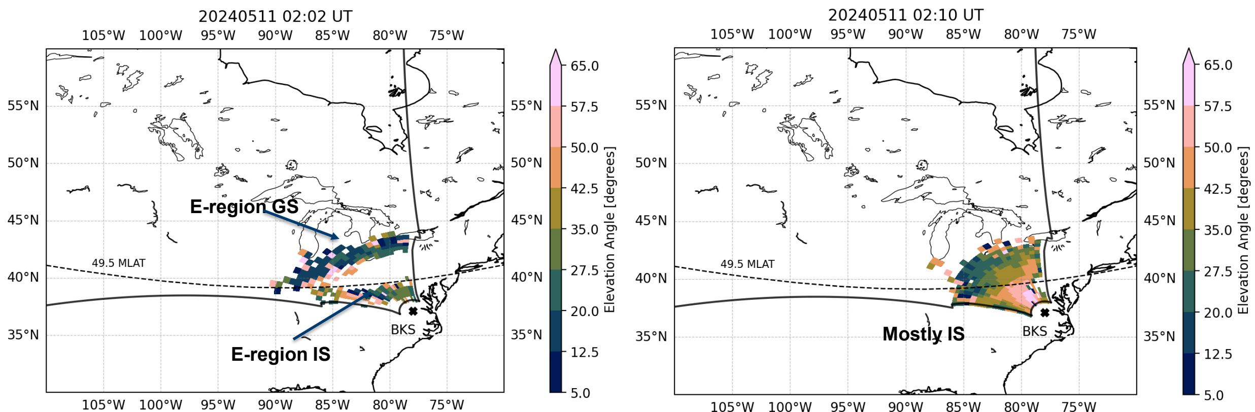
Backscatter from a broad range of elevation angles ( $20^\circ$ - $55^\circ$ ) than normal, including very high one's ( $\geq 50^\circ$ ), is observed during the interval. There is an overall trend for elevation angle to drop with range. The high elevation angle backscatter corresponds to unusually high virtual heights (>250-300 km) at near ranges.
